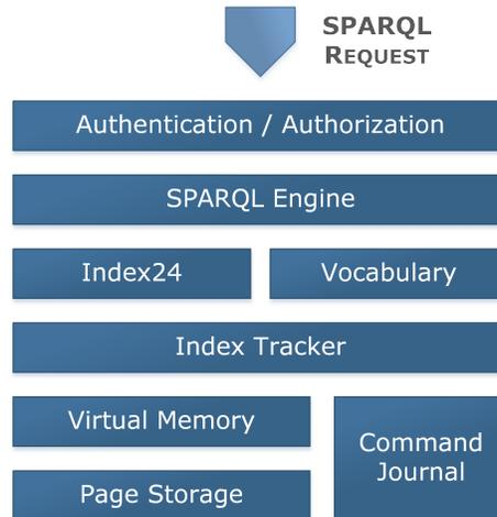
**Fig. 1.** Architectural design of QUAD.
